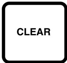
The **CLEAR** key is used to erase an erroneous entry, and return the cursor back to the first character in the entry field.
