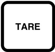
The **TARE** key is used to enter a known tare (container) weight via the numeric keypad. Pressing the TARE key will display zeros or the previously entered tare (if any) and illuminate the TARE annunciator.
