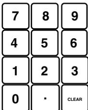
The **NUMERIC KEYS** are used to enter numeric values required in the various operational modes and calibration procedures of the scale. The 1 and 0 keys are also used to answer YES and NO questions displayed in certain operations. The 1 and 2 keys are also used to select between scale #1 (local) and scale #2 (remote).
