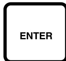
The **ENTER** key is used when keying in some calibration and operational data, to accept or terminate the entry.
