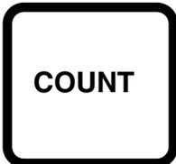
The **COUNT** key is pressed after removing or adding the sample requested, to initiate the counting operation and place the display in the **COUNT** mode. The **COUNT** key will return the display to the count mode from any weight display or sample mode.
