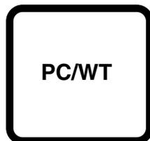
Pressing the **PC/WT** key will display the calculated number of pieces per pound. This number is calculated as the reciprocal of the WT/PC value. The PC/WT annunciator will illuminate.
