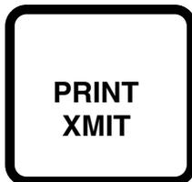
Pressing the **PRINT XMIT** key will transmit RS-232 data to an optionally installed printer, printing data which is currently shown on the scales display, along with descriptive headings. See section 6.0 for further information.
