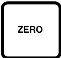
Pressing the **ZERO** key with weight on the scale, will set the gross weight to zero, and clear the tare weight, if any. If the display is in count mode, the count will be set to zero.
